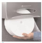
1 Install new roll by aligning "dimple" in center of tissue roll with left arrow located on the lower left of the dispenser front. With tissue unrolling in clockwise direction, push roll upwards firmly until it snaps into place.
