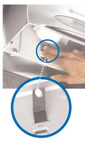
3 When the tissue roll is no longer visable through the viewing window, the roll may be transferred to the stub roll holder. To remove main roll, slip hand upward between back side of the roll and the front side of the metal spring. Depress the metal spring slightly and dislodge the roll. Pull down easily to remove.
